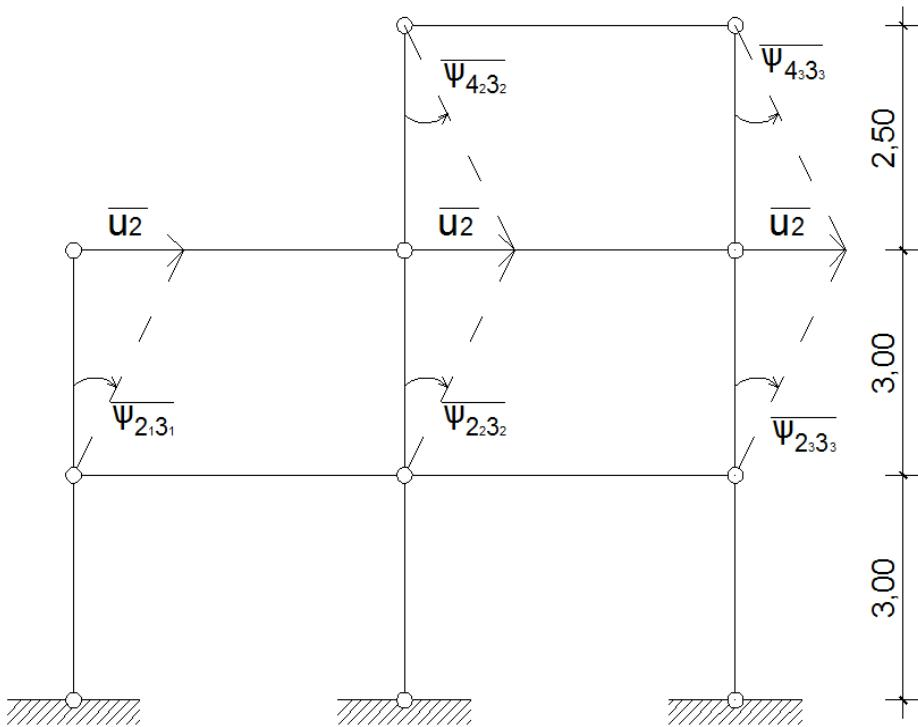
$$\overline{\Psi_{2_13_1}} = \overline{\Psi_{2_23_2}} = \overline{\Psi_{2_33_3}} - \frac{u_2}{h_2} = -\frac{100}{3,0} = -33,33$$
