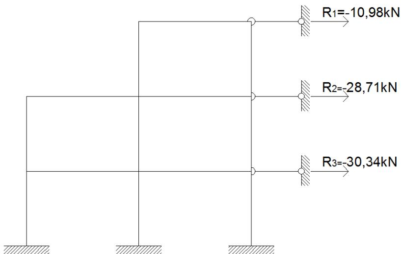
$$H_1 = R_1 = 10,98\text{kN}$$
