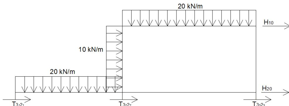
$$T_{3_12_1} = \frac{10 \cdot \frac{3^2}{2} - 7,6 + 11,9}{3,0} = 16,33 \text{ kN}$$
