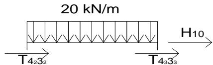
$$T_{4_23_2} = \frac{10 \cdot \frac{2,5^2}{2} + 22,2 - 1,1}{2,5} = 20,94 \text{ kN}$$
