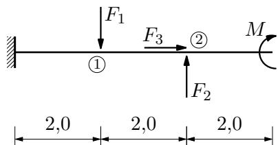
$$\begin{aligned}F_1 &= 120,0 \text{ kN} \\F_2 &= 50,0 \text{ kN} \\F_3 &= 100,0 \text{ kN} \quad (\text{na osi grede}) \\M &= 50,0 \text{ kNm}\end{aligned}$$
