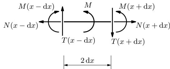
$$-N(x-dx) + N(x+dx) = 0 \quad \Rightarrow \quad \boxed{N(x-dx) = N(x+dx) = N(x)}$$
