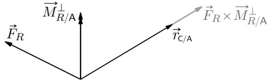
$$\vec{F}_R \perp \vec{M}_{R/A}^\perp \implies \|\vec{F}_R \times \vec{M}_{R/A}^\perp\| = \|\vec{F}_R\| \|\vec{M}_{R/A}^\perp\|$$
