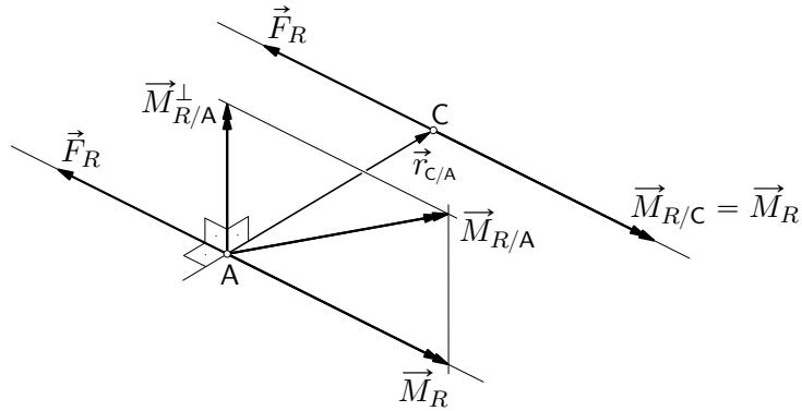
$$\vec{M}_{R/A} = \vec{M}_R + \vec{M}_{R/A}^\perp \implies \vec{M}_{R/A}^\perp = \vec{M}_{R/A} - \vec{M}_R$$
