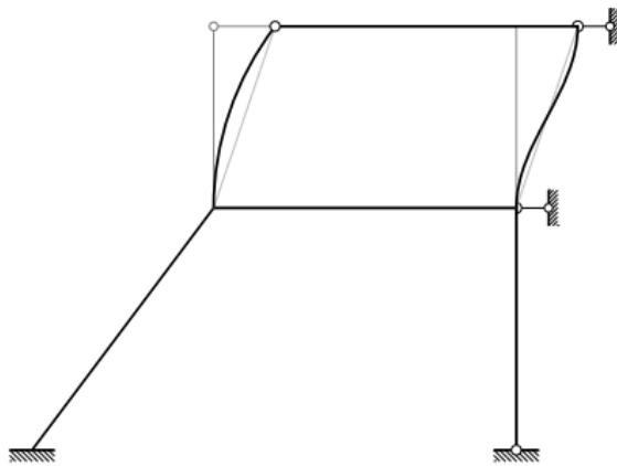
$$\overline{M}_{3,5} = -3 k_{\{3,5\}} \overline{\Psi}_{\{3,5\}} = -3 \frac{EI}{3} \left( -\frac{33,3}{EI} \right) = 33,33$$
