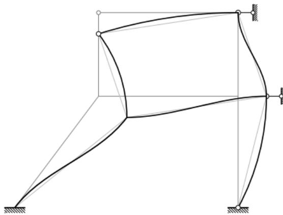
$$\overline{M}_{4,6} = \overline{M}_{6,4} = -6 k_{\{4,6\}} \overline{\Psi}_{\{4,6\}} = -66,7$$
