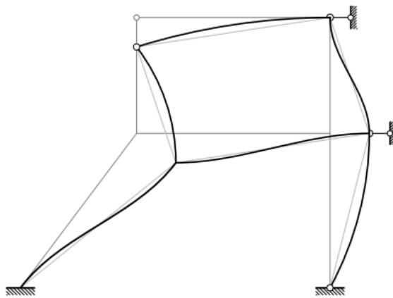
$$\overline{M}_{1,3} = \overline{M}_{3,1} = -6 k_{\{1,3\}} \overline{\Psi}_{\{1,3\}} = 30,0$$
