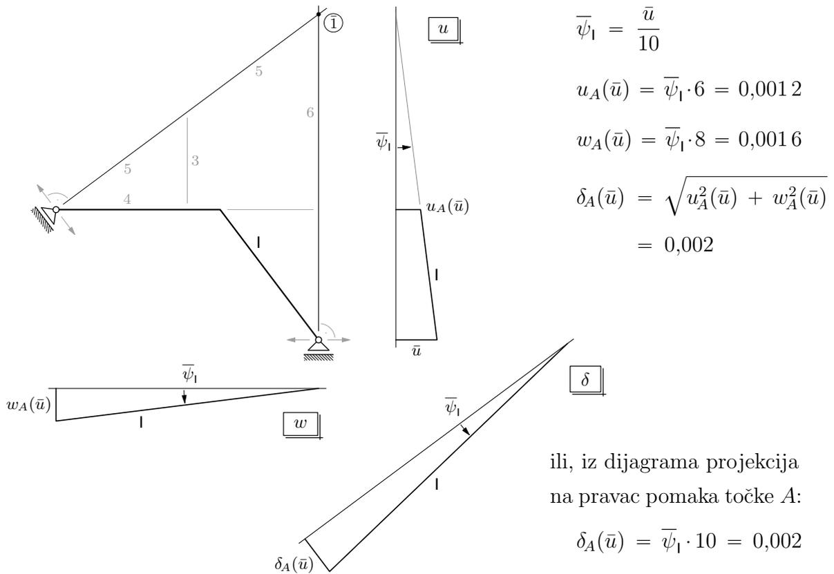
$$\delta_A = \delta_A(M) + \delta_A(\bar{u}) = -0,000\,061\,471\,2 + 0,002 = 0,001\,938\,53 \text{ m} = 1,94 \text{ mm}$$
