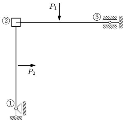
$$\begin{aligned} \overline{M}_{2,1}^{(c)} &= \overline{M}_{2,1} - \frac{1}{2} \overline{M}_{1,2} = -\frac{P_2 \ell_{\{1,2\}}}{8} - \frac{1}{2} \frac{P_2 \ell_{\{1,2\}}}{8} \\ &= -\frac{3 P_2 \ell_{\{1,2\}}}{16} = -\frac{3 \cdot 50 \cdot 4}{16} = -37,5 \text{ kNm} \end{aligned}$$
