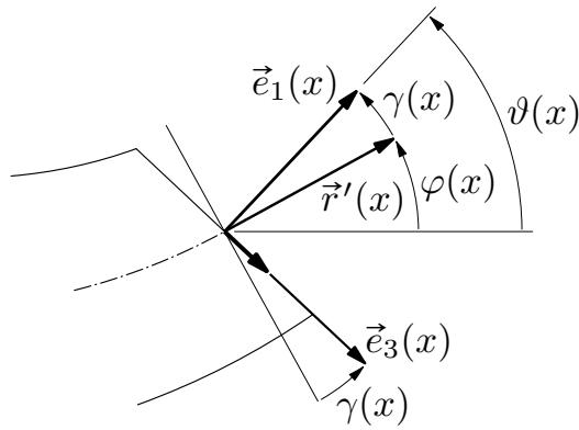
$$\vartheta(x) = \varphi(x) + \gamma(x) = -w'(x) + \gamma(x)$$
