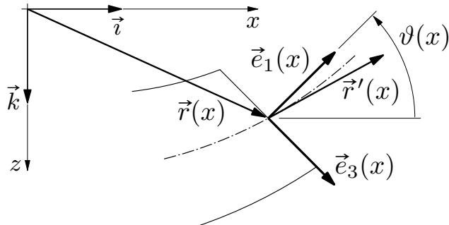
$$\vec{r}(x) = [x + u(x)] \vec{i} + w(x) \vec{k} \quad \text{or} \quad \vec{e}_1(x)$$
