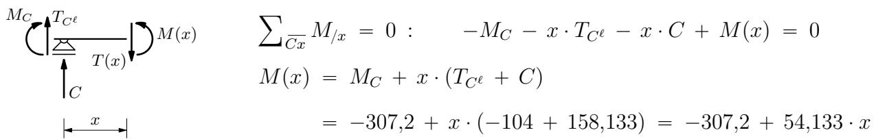
$$M(0) = -307,2 \text{ kNm} = M_C \quad \not\propto \quad M(3,2) = -133,974 \text{ kNm} = M_H$$
