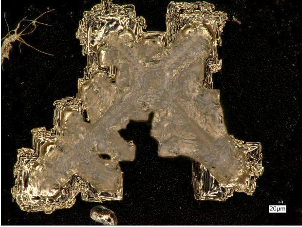
Figure 7: When the focal plane of a microscope sweeps through the object, this is equivalent to a perfectly controlled translation of the object along the optical axis. The single pictures do not have to be registered – they are all scaled in the same manner.
