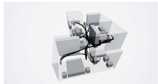
Figure 13: Perspective view of the AI calculated flows considering furniture
