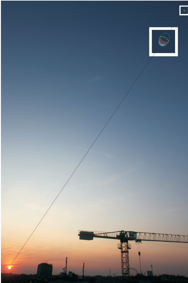
Figure 6: Photo with 20 mm focal length (optical angle about 90^\circ ). Despite extremely high resolution (22 megapixel) the moon (top, right) also appears blurred in the magnification (framed white) due to the small size in the picture, but obviously elliptically distorted.
